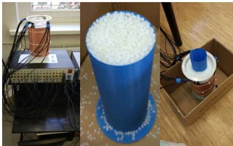
Fig. 5. The main components of the experimental setup used in this study – a measurement system and two 3D printed test phantoms filled in PE granulate.
