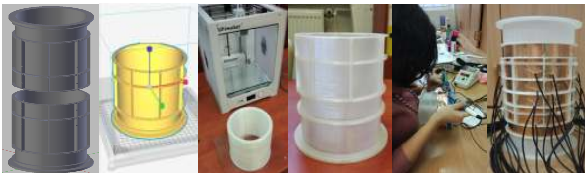
Fig. 3. The main steps of modelling, design and finishing 3D printed ECT sensor.
