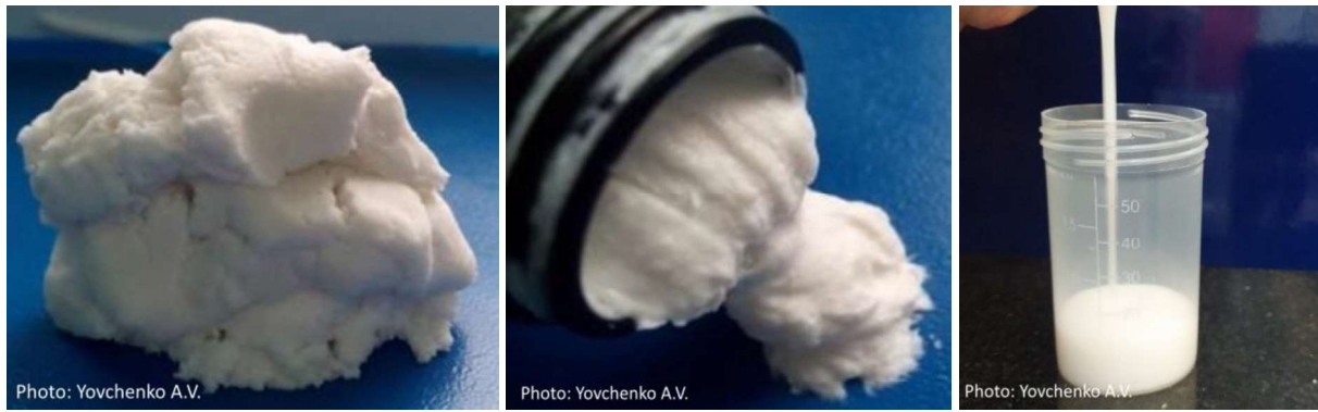
a) pasty PCS (45 % paraffin, 45 % water, 10 % SAA (Tween 60:Span 80, 1:1)); b) gel-like PCS (25 % paraffin, 65 % water and 10 % SAA (Tween 60:Span 80, 1:1)); c) liquid PCS (25 % paraffin, 70 % water and 5 % SAA (Tween 60:Span 80, 1:1)) Fig. 5. Photos of PCSs “paraffin in water” after 6 months of storage.
